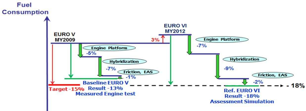
Figure 3: The diagram shows the achieved CORE results of reduced CO<sub>2</sub> by improved powertrain efficiency.
