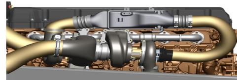
New design of two stage turbo applied on the engine
