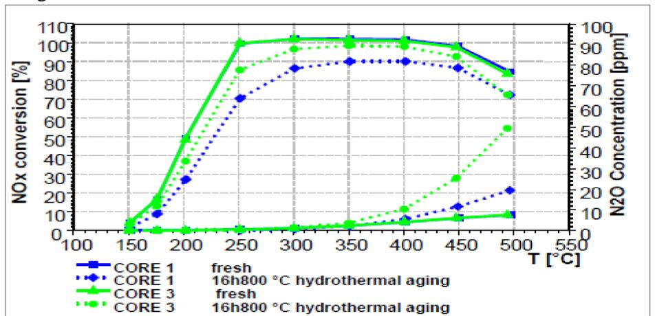
Improved low temperature performance with new SCR coating
